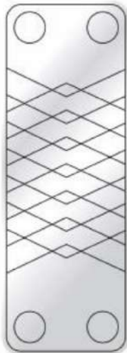
D通道 Passage D A channel consisting of large Angle corrugated plates
