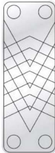
H通道 Passage H A channel consisting of a mixture of large and small Angle corrugated plates
