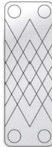
X通道 Passage X A channel consisting of small Angle corrugated plates
